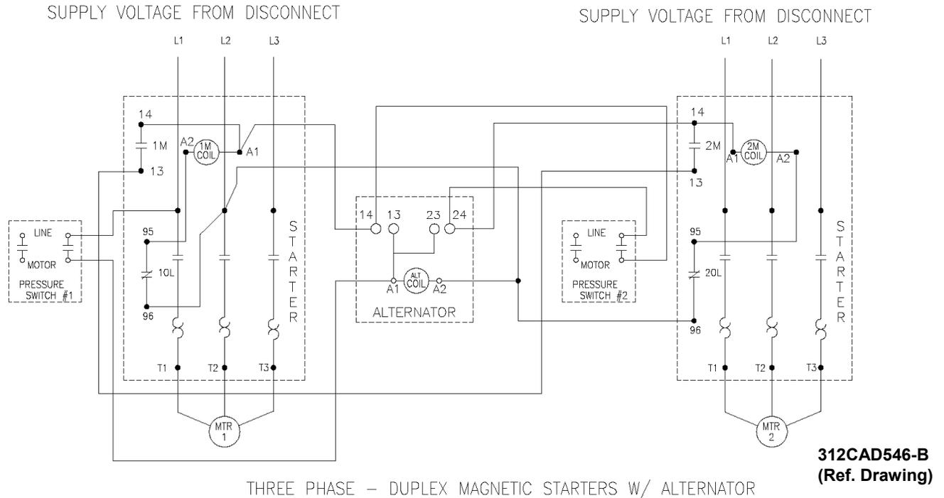
**Figure 1-2 Duplex Wiring Diagram**
