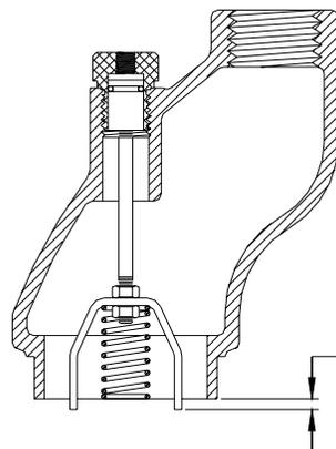
WHEN INSTALLING HEAD UNLOADER MAINFOLD ASSEMBLY, BE CERTAIN THAT THE ACTUATING CLAW PROTRUDES 3/16" BELOW THE BOTTOM OF THE MANIFOLD. CLAW MUST BE POSITIONED SO THAT IT WILL ENTER TWO SLOTS IN THE COMPRESSOR VALVE. FAILURE TO FOLLOW THIS PROCEDURE WILL RESULT IN AN INOPERATIVE HEAD UNLOADER.
