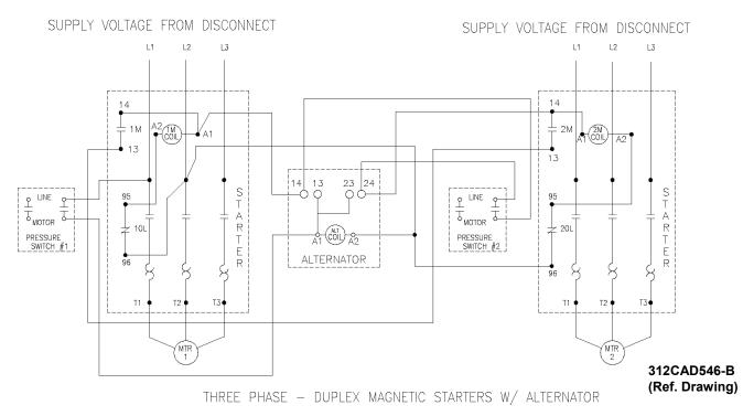
Figure 1-2 Duplex Wiring Diagram
