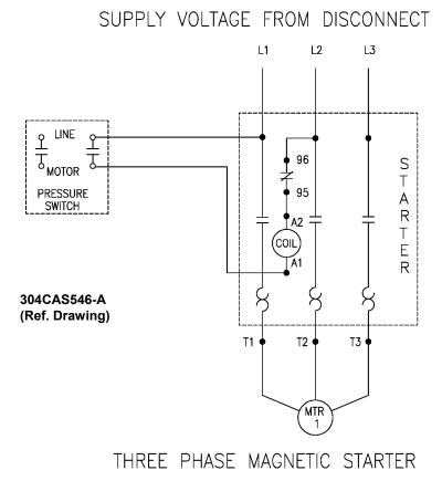
Figure 1-1 Simplex Wiring Diagram
